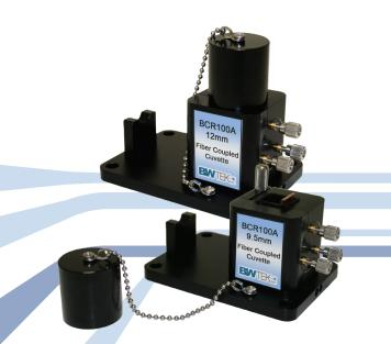
BCR100A series cuvette holders are designed for raman sampling. The BCR100A holds a standard 12.5 x 12.5 mm cuvette for Raman measurement of a liquid or powder sample. The cuvette holder is designed to work with B&WTek, Inc. Raman probes and provides a stop to prevent the probe shaft from hitting the cuvette and an excitation light trap to reduce background fluorescence.
